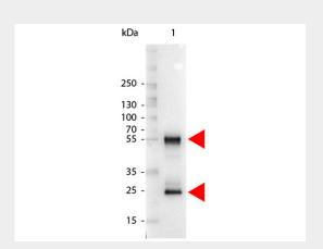
Western Blot of Alkaline Phosphatase Conjugated Rabbit anti-Mouse IgG antibody. Lane 1: Mouse IgG. Lane 2: none. Load: 100 ng per lane. Primary antibody: none. Secondary antibody: Alkaline Phosphatase mouse secondary antibody at 1:1,000 for 60 min at RT. Block: MB-070 for 30 min RT. Predicted/Observed size: 55 kDa, 28 kDa for Mouse IgG. Other band(s): none.
